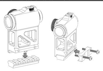
Place the YORK SOM with the optic installed on the desired position on the top rail.
